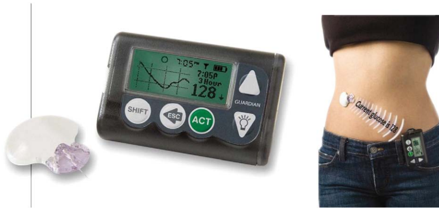
Fig. 2. Real time continuous glucose monitoring device. Sensor attached to transmitter next to real time monitor displaying 3-hour glucose profile (mg/dl) and demonstrated in situ in an adult. Images provided by Medtronic Ltd.
